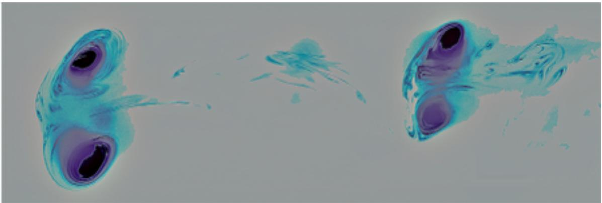
The image seen above was taken in an attempt to reveal details of the beauty and complexity within a ring of fog. The intension of this image was to clearly show the internal shear layers forming vortex lines on a cross sectional field of view. The swirling motion shown is the direct result of how a fog ring manages to move consistently through space.
